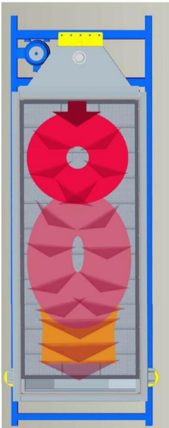
When material fall into the inlet of the M series gyrotary screener, the baffle and distributor will distribute the material materials first,the material movement is the reciprocating gyrotary motion
