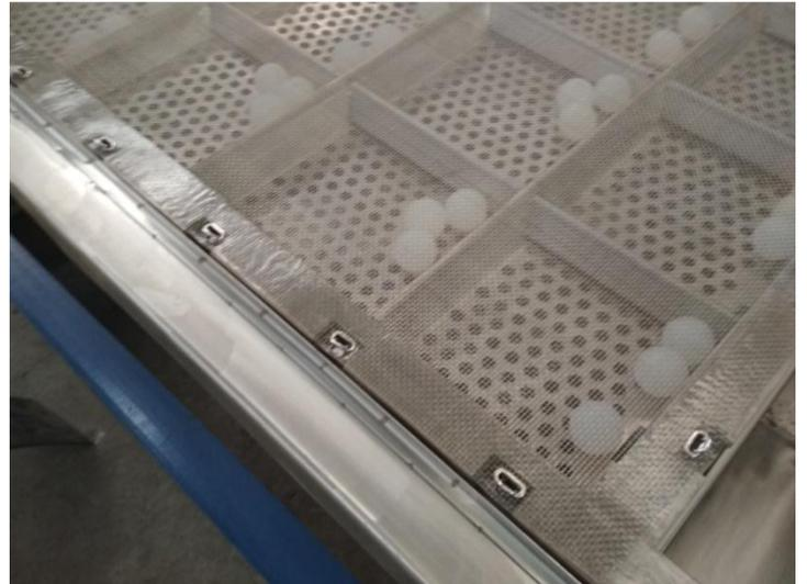
The gyrotory screener deck is one combination structure that consist of screener mesh , self-cleaning ball and support deck frame.
