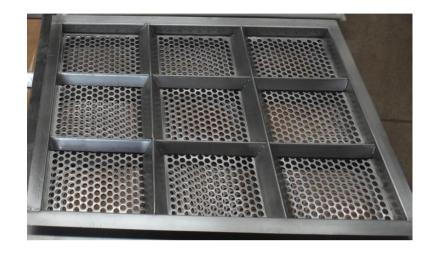
The side door gyratory screener deck is one combination structure that consist of screener mesh, self-cleaning ball and support deck frame. The screener mesh be fixed on screener ball tray directly.
