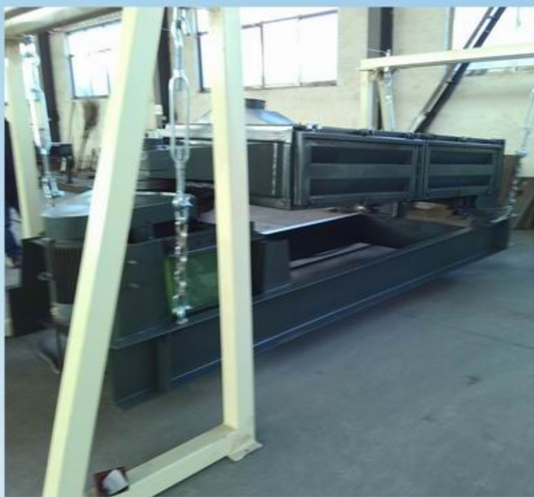
MGP Gyrotory Screener Test running in workshop
