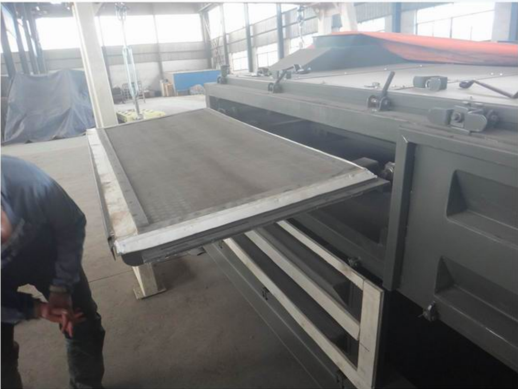
The screener panel width usual is the 1/2 of screener equipment width, the screener pannel length is the 1/2 to 1/4 of the screener equipment length, it save more installation room.
