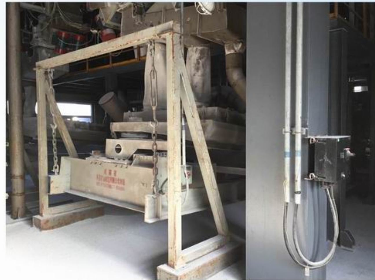
Screener MP-SE36 (right) For Screening wheat at site
