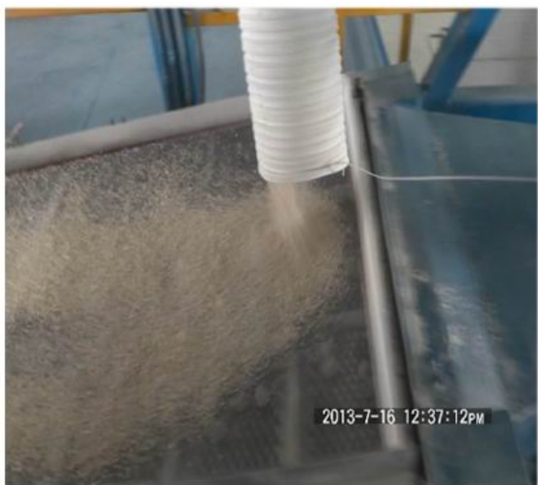
Stage 1 Material distribute at inlet
