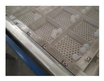
The gyratory screener deck is one combination structure that consist of screener mesh , self-cleaning ball and support deck frame. The screener mesh be fixed on screener deck frame via spring clamp.
