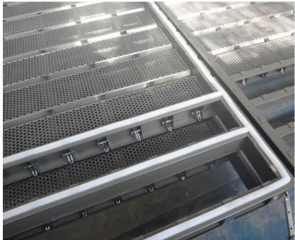
**Replaceable seal of the screener deck**
