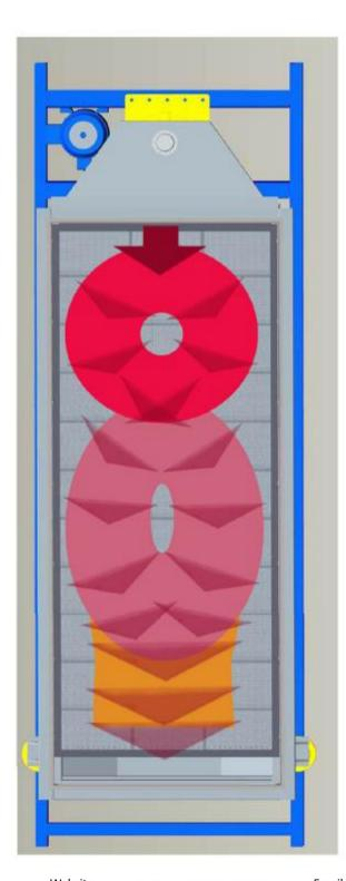
When material fall into the inlet of the M series gyratory screener, the baffle and distributer will distribute the material materials first, the material movement is the reciprocating gyratory motion
