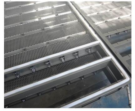
Replaceable seal of the screener deck
