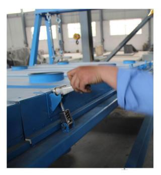
The fast clamp for top cover is adjustable, and it is easy to open and fasten
