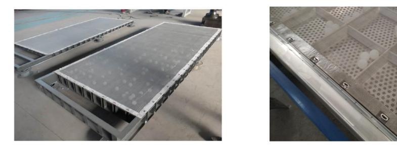
The gyratory screener deck is one combination structure that consist of screener mesh , self-cleaning ball and support deck frame. The screener mesh be fixed on screener deck frame via spring clamp.
