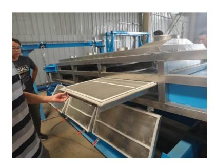
Replaceable seal of the screener deck
