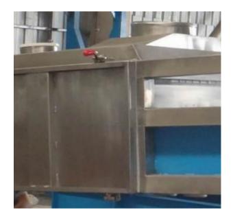
This model clamp is one standard parts, the customer could open and close the side cover in short time
